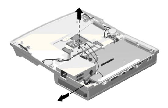
Figure 6-12. Disconnecting the Power Supply
